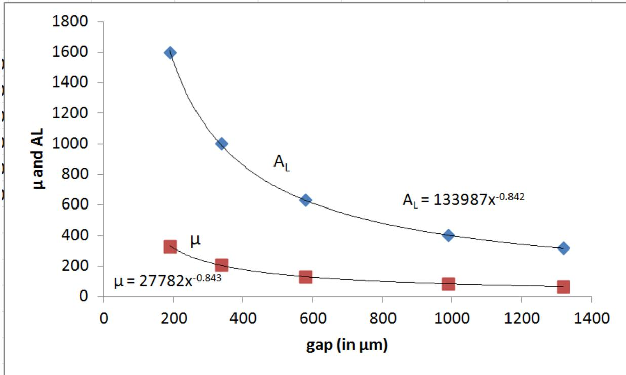
Figure 7.37: TRENDLINE of 4229 Pot core AL values and effective permeability
