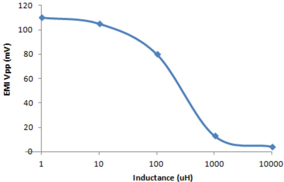
Figure 7.29: EMI as a function of series line inductor for the 10W load of Figure 7.46
