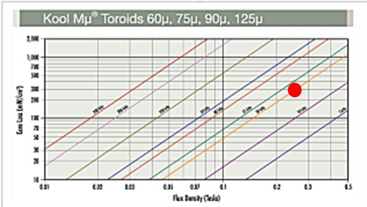
Figure 7.23: Sendust core loss chart
