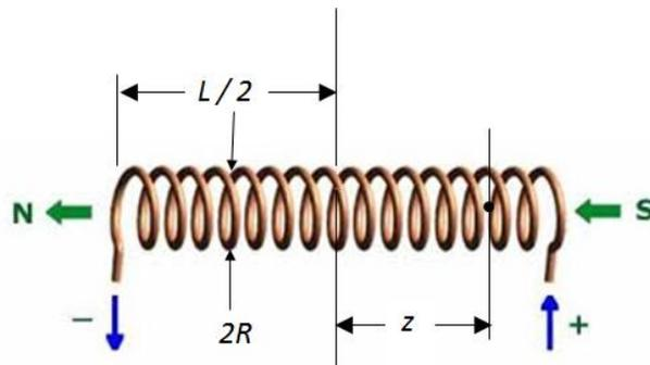
Figure 7.2: Long solenoid inductor
