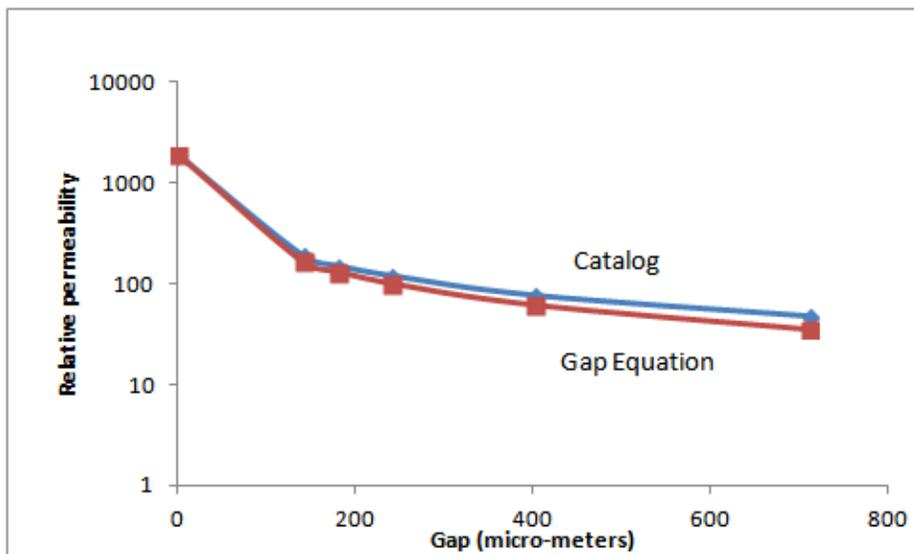
Figure 7.12: Values of effective permeability from catalog and from equation
