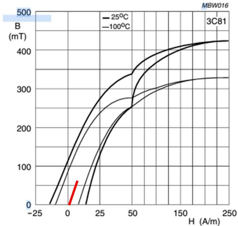
Figure 7.24: Maximum BH curve for 3 Watt converter
