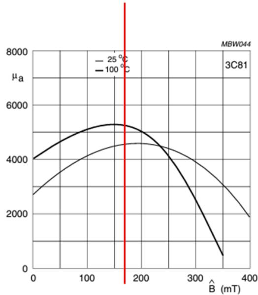
Fig.4 Amplitude permeability as a function of peak flux density.
