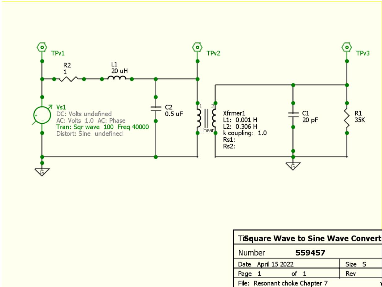
Figure: 7.33: Square wave to sine wave converter
