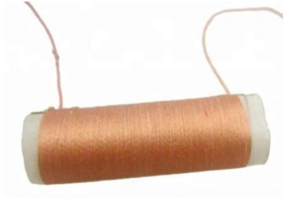
Figure 7.3: Air-core paper-towel tube solenoid
