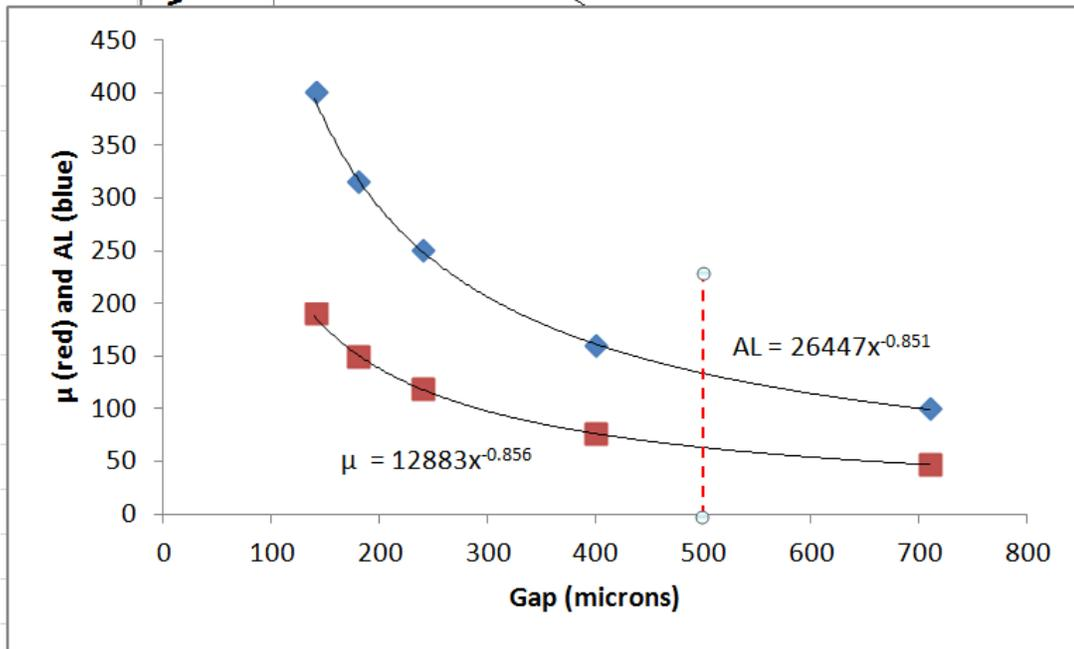
Figure 7.9: Effective Gap Permeability and  $A_L$  as a function of gap using data points from the catalog
