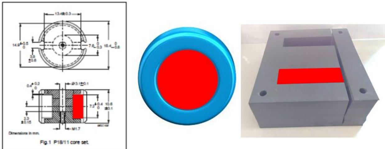
Figure 7.13: Winding area  $W_a$  of different cores (in red)
