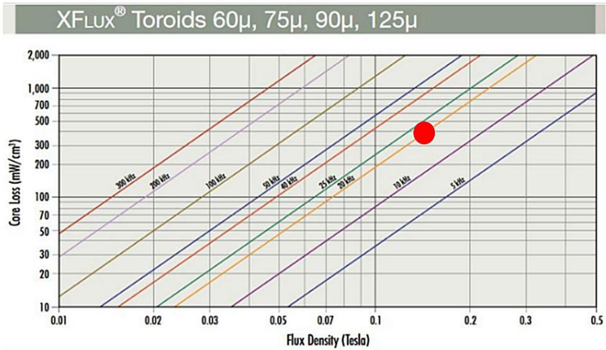
Figure 7.21: Powdered iron loss chart
