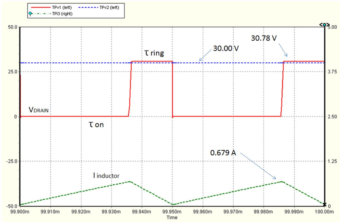
Figure 7.15: 9 to 30V ringing choke converter
