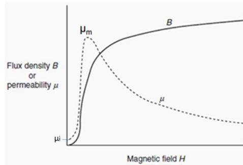
Figure 7.5: Permeability vs H field
