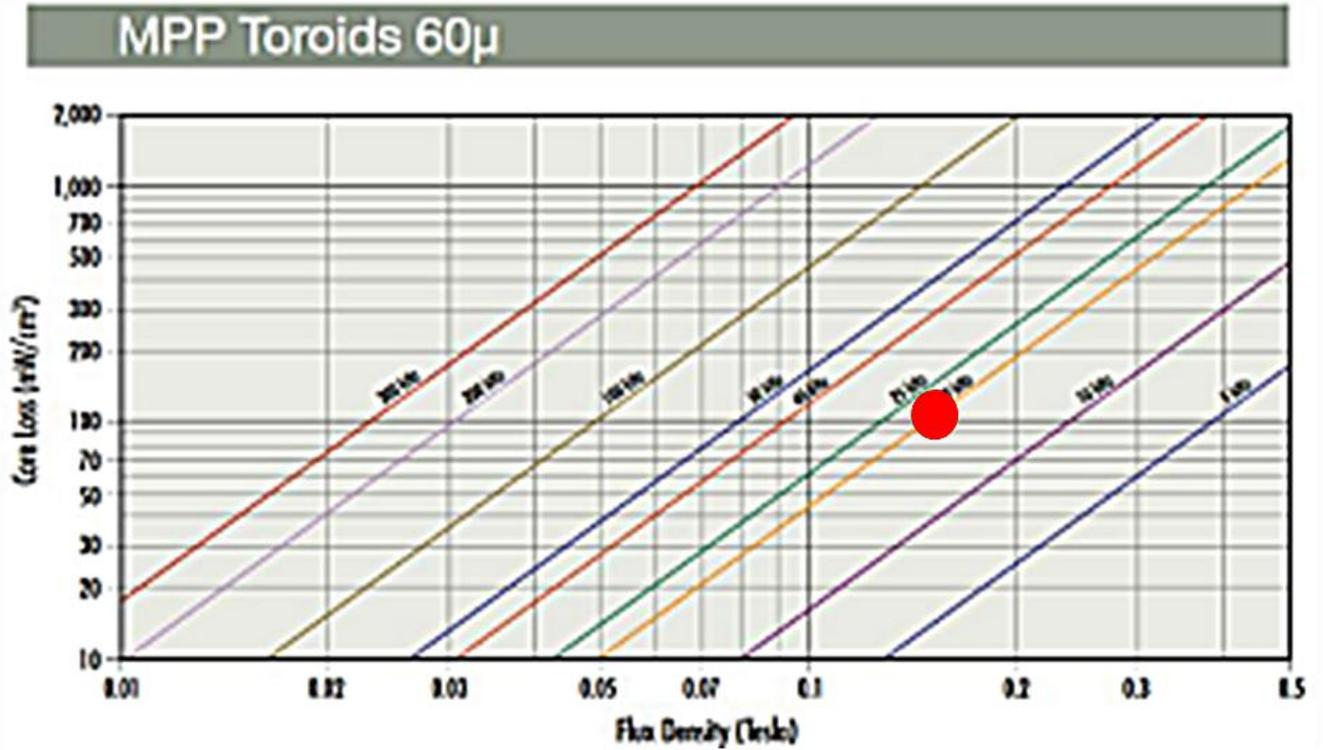
Figure 7.22: MPP Core loss chart
