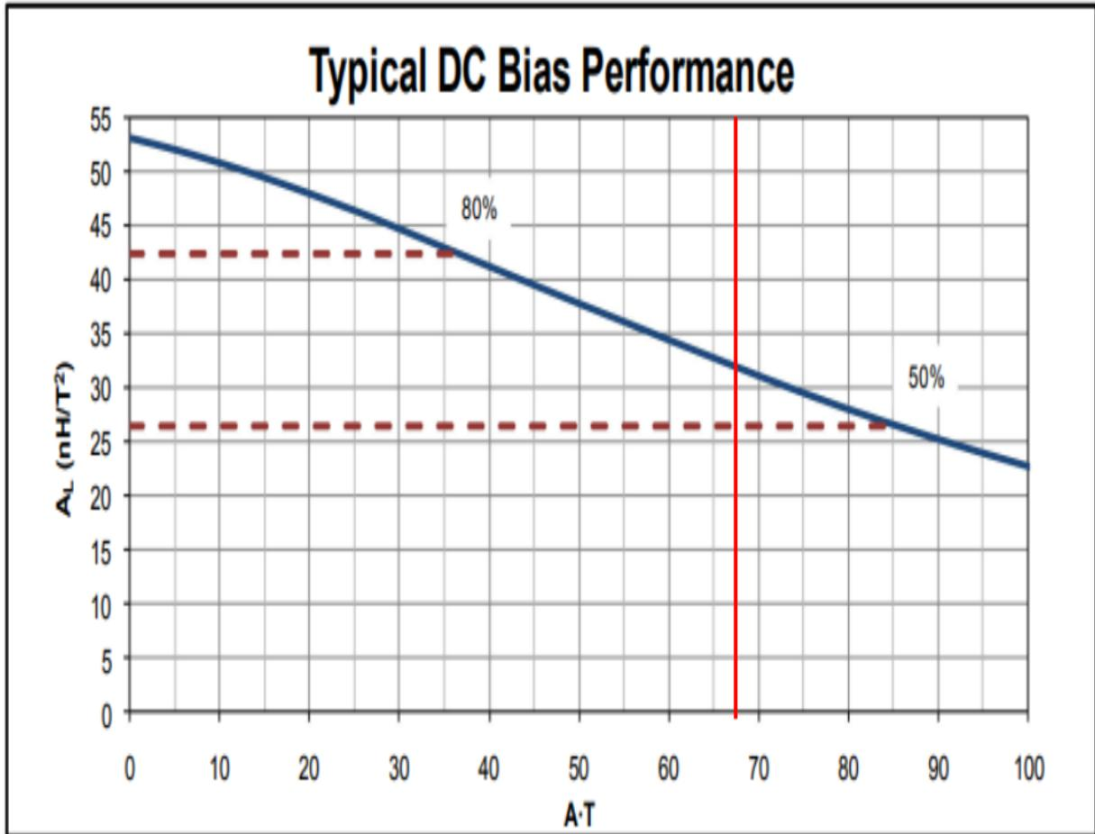
Figure 7.27: Sendust core inductance drop-off
