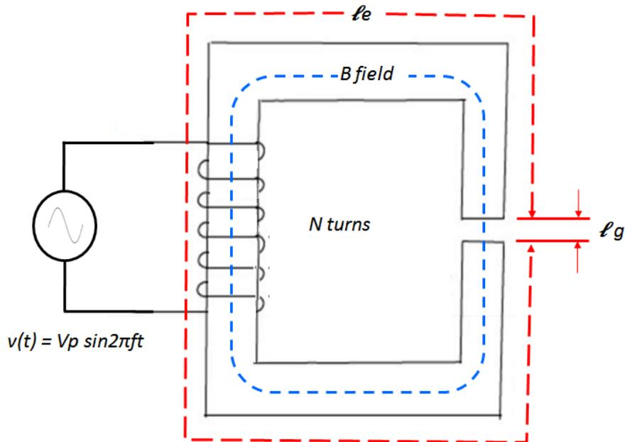
Figure 7.10: Ferrite core of physical length  $\ell_e$  with gap  $\ell_g$
