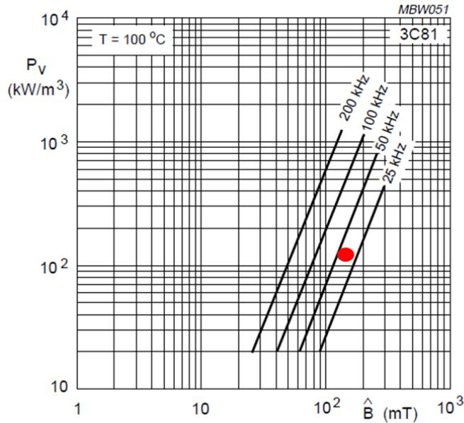
Figure 7.38: Resonant choke core loss 3C81
