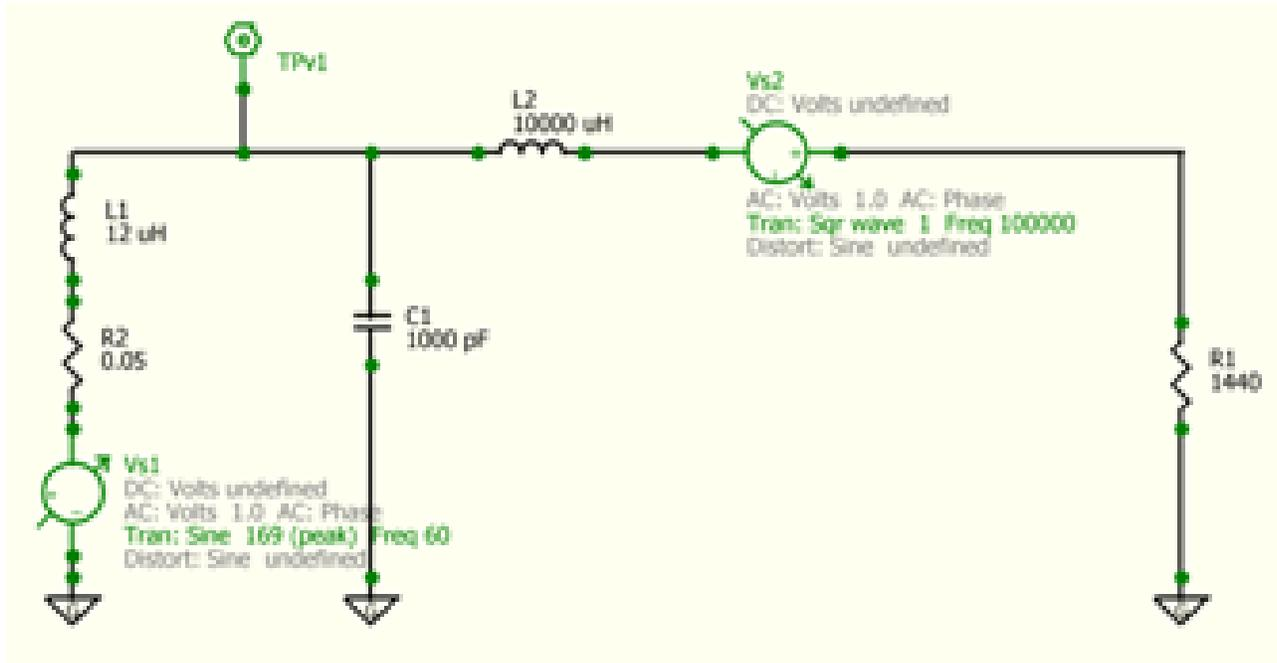
Figure 7.28: SPICE test circuit for EMI reduction
