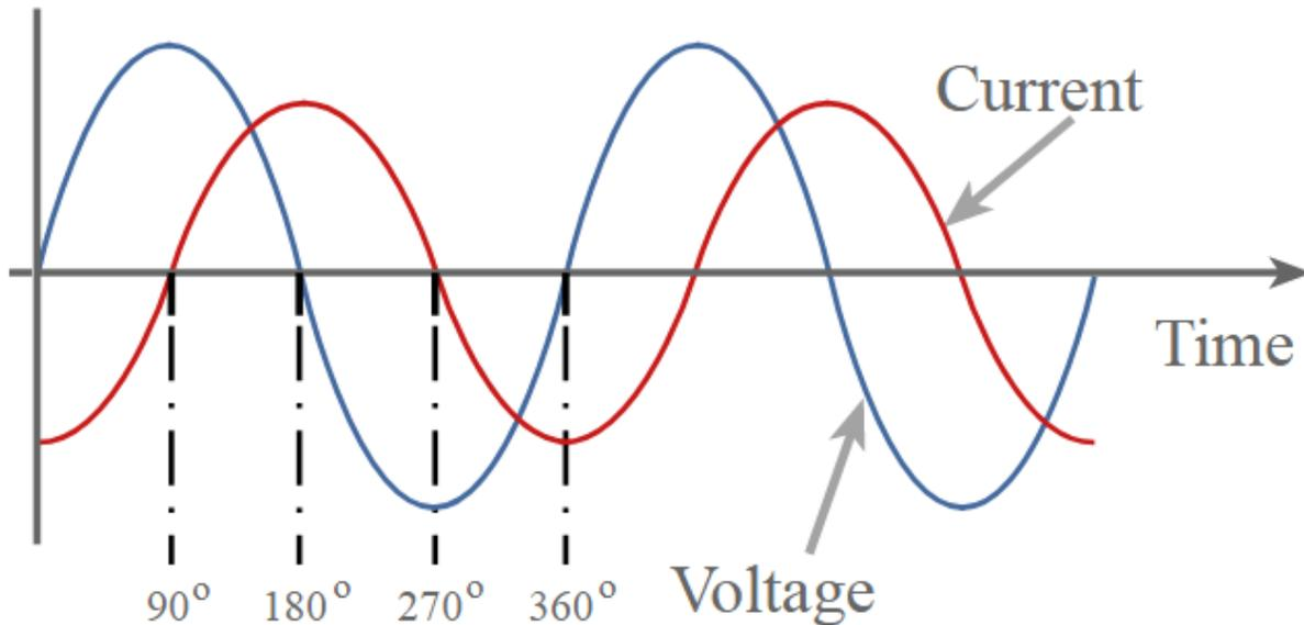
Figure 7.11: Voltage and resultant current waveforms (electronics-notes.com)
