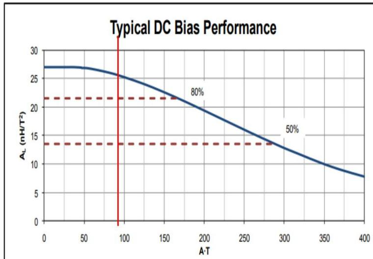
Figure 7.26: AL drop off as a function of current in the C0055051A2 MPP core
