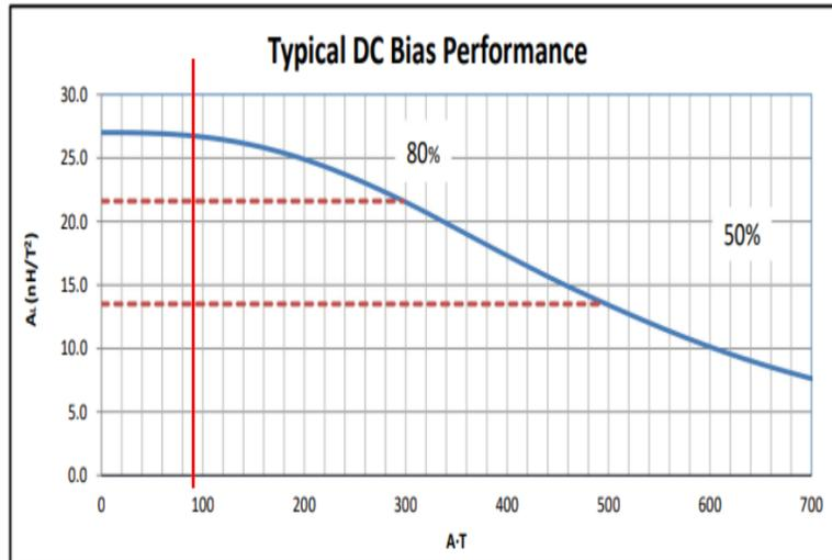
Figure 7.25: AL drop off as a function of current in the 78051A7 iron powder core
