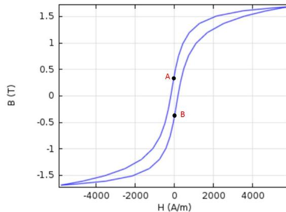
Figure 6.12: BH Loop silicon steel
