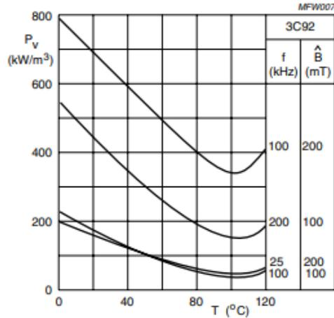
Figure 6.13: Hysteresis loss as a function of temperature.
