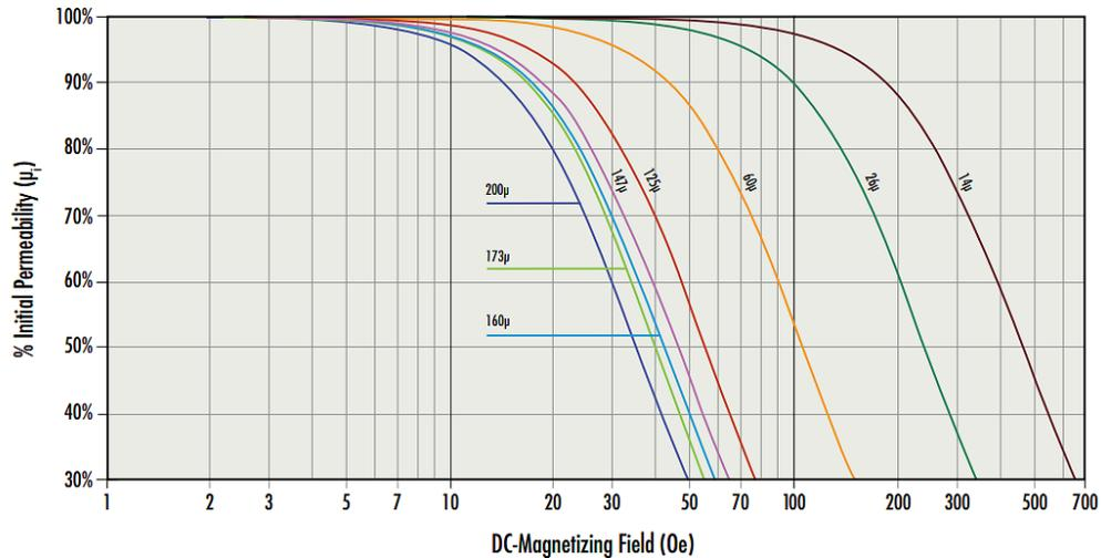
Figure 6.10: Permeability as a function of DC magnetizing field for MPP core material
