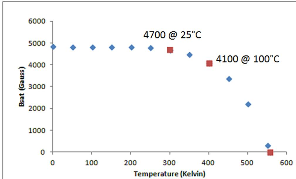
Fig: 6.11: Bsat for 3C92 ferrite material
