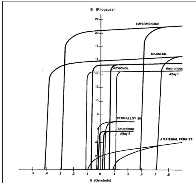
Figure 6.8: BH curves for various ferromagnetic materials (Magnetics)
