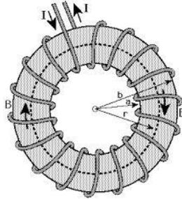
Figure 6.3: Toroidal inductor wound on plastic form
